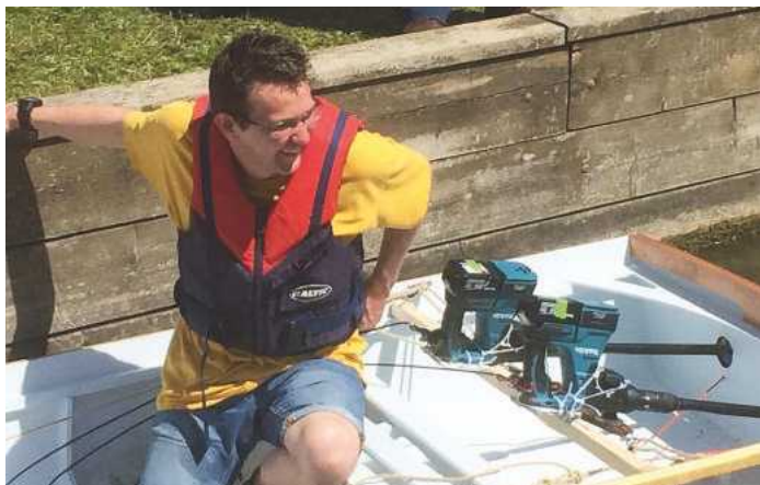
Simon Smith in Pagan, powered by two Makita DHR243 18V brushless rotary hammer drills, pictured, won Makita's Cordless Tender Challenge in which contestants in boats under 10ft had to pick up a passenger and ferry her/him back to the start. The winner of the Canoe Challenge was Adam Brown in a craft powered by two DHP4546 18V combi drills
